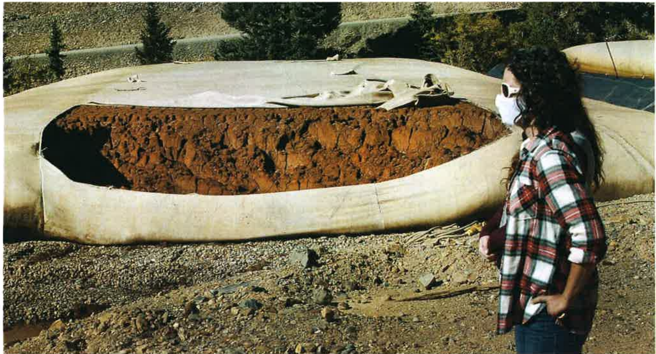
A bladder holds solids in 2020 at the Gold King water-treatment plant that have been collected from the water flowing out of the Gold King Mine. (Jerry McBride/Durango Herald file)
