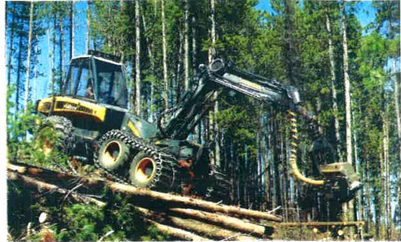
The Ponsse Ergo Harvester, a steep-slope extractor, made its Colorado wildfire mitigation debut last year on the Peak 7 forestry project, removing lodgepole pine above Breckenridge neighborhoods. Built like a tractor with robotic arms, the harvester can traverse steep inclines with minimal impact on the ground to cut trees, strip branches and stack logs for removal. “In the past, a project like this would have required a helicopter, which was expensive, or a hand crew,” said Bill Wolf, a Colorado State Forest Service forester. Photo: Denver Water
