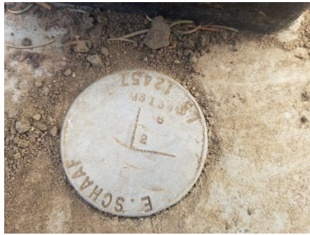
Gate damaged by snow creep Survey pin in post foundation
