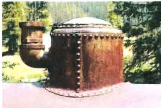
Dome with breather valve – 21-in. diameter
