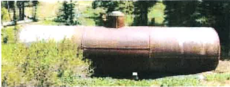
Tank side and quarter views – 24-ft long, 5-ft 7-in. diameter. Three courses of 0.25-in. steel plate; pointed rivets 2-in. apart. Welds and marks for old hand grabs, hand rails, and straps.
