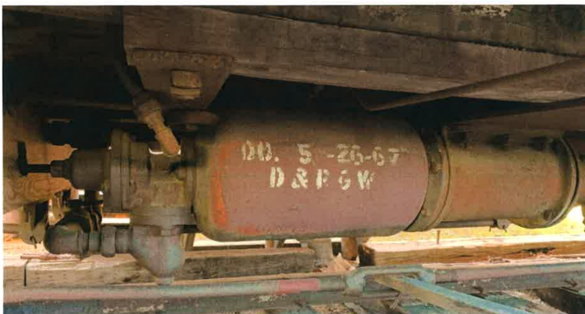
Two photos of Boxcar 3101 at 855 CR 18, Gunnison. Printed on the air reservoir is evidence that the car was in Durango on 26 May 1967. —Leighton Moreland
