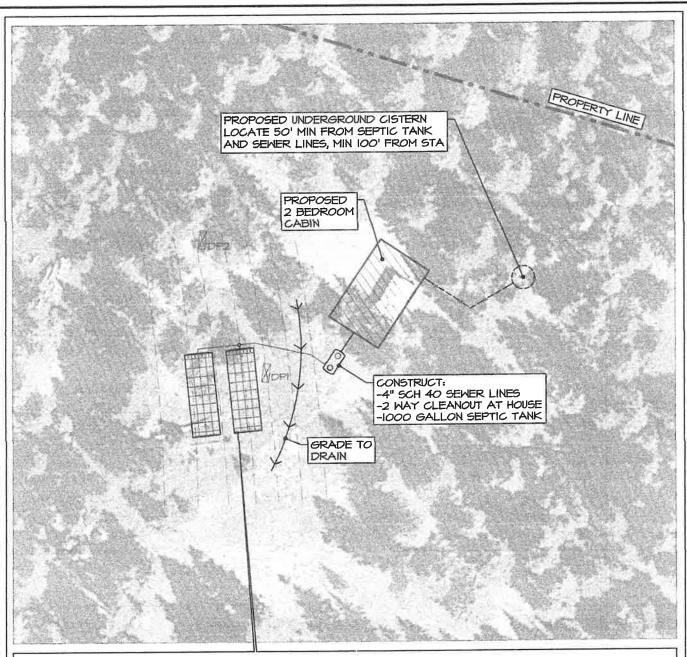
CONSTRUCT NEW SOIL TREATMENT AREA (STA): PROVIDE 864 SQ FT OF BED AREA.
