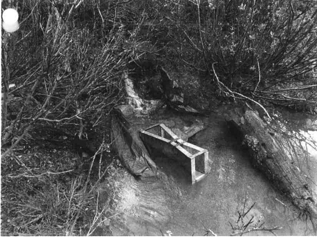
Adit Discharge volume location. Discharge was gathered (during measurement) into a 1-inch portable Parshall flume was utilized for accuracy.
