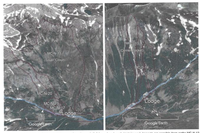
Figure 7. Avalanche paths affecting the lodge area from the north (left image) and south (right image). Impacts are possible from paths MC-N-13 (Silver Cloud), MC-S-13 (Corner Pocket), MC-S-14, MC-S-15, and MC-N-20. Design avalanches from MC-N-17, and -19 could result in dense flow overtopping the lodge and impacting the lodge area immediately to the east of the buildings.
