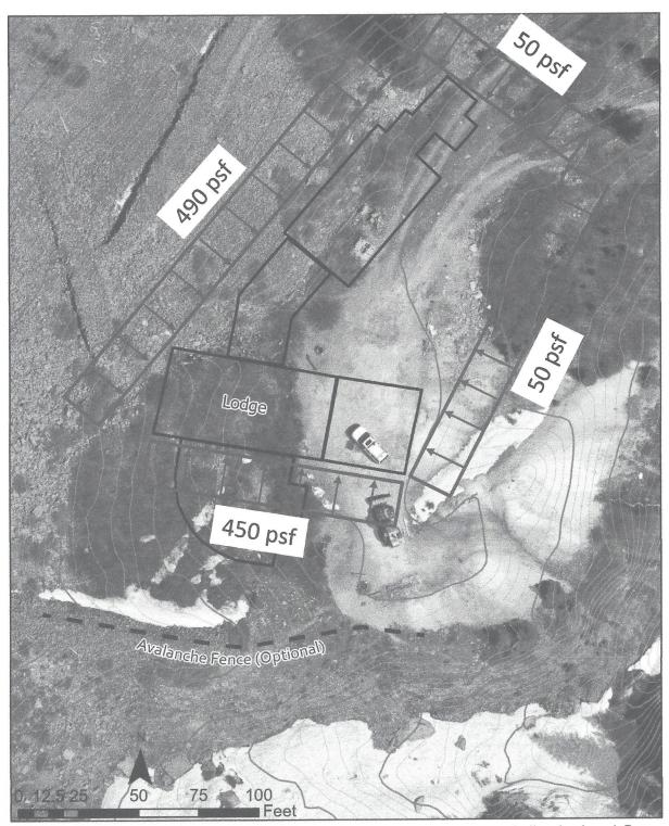
**Figure 1.** The lodge area in plan view (1:500 scale) with annotated loads from each direction in red. Dense flow loads are applied from the south and west. A powder flow load of 50 psf is applied from all directions. A draft building footprint is shown in black. The centerline of the optional avalanche fence is also shown.
