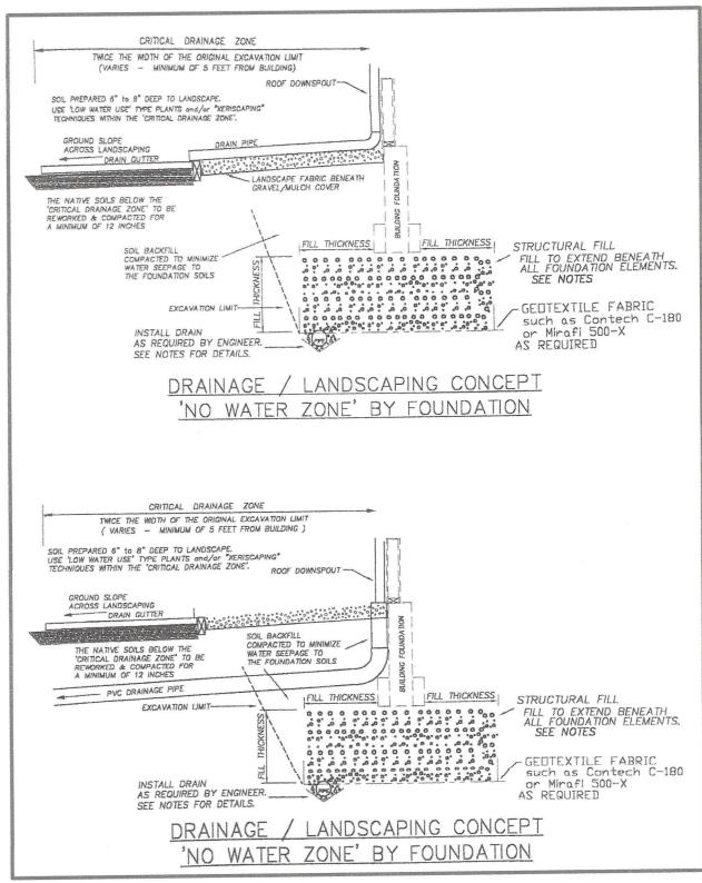
Figure 7. Example Downspout Drains to Carry Water Away from the Foundation.
