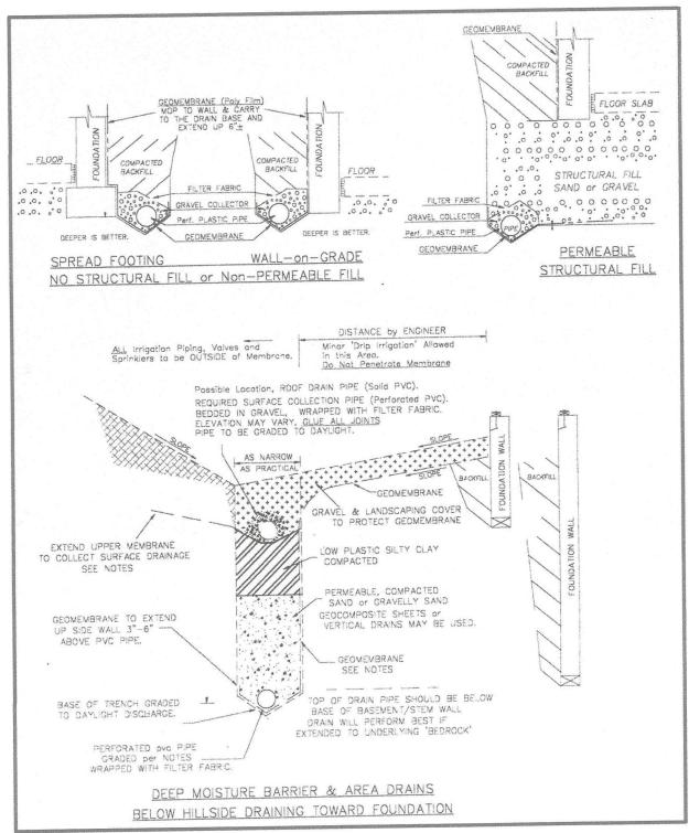
Figure 8. Example Foundation Drains to Carry Water Away from the Foundation.
