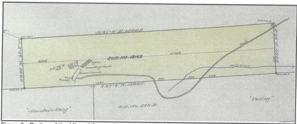
Figure 3. Portion of the Mineral Survey Plat for the Shelbyville Lode (MS 18168) showing the improvements made at the Silver Crown Lode as of November 1906.
