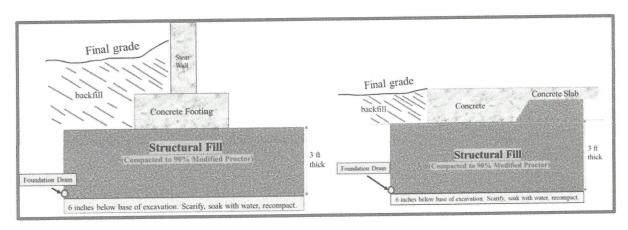
Figure 5. Schematic of the Foundation Designs for Surface Facilities. The Same Schematic Applies to Pads for Concrete Piers.
