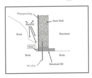
Figure 6. Schematic of the Surface Facilities Connection to Bedrock (where applicable).
