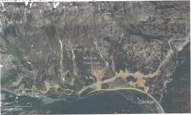
Figure 4. Three large avalanche paths which produce Size D3 avalanches which reach the lower switchback of Highway 550 every 1-3 years. Access between the garage and lodge in yellow.
