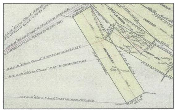
Figure 59. Portion of the October 1906 plat for MS 18179 showing the Milwaukee Lode and its discovery cut and tunnel. Note that no road is shown running through the claim.
