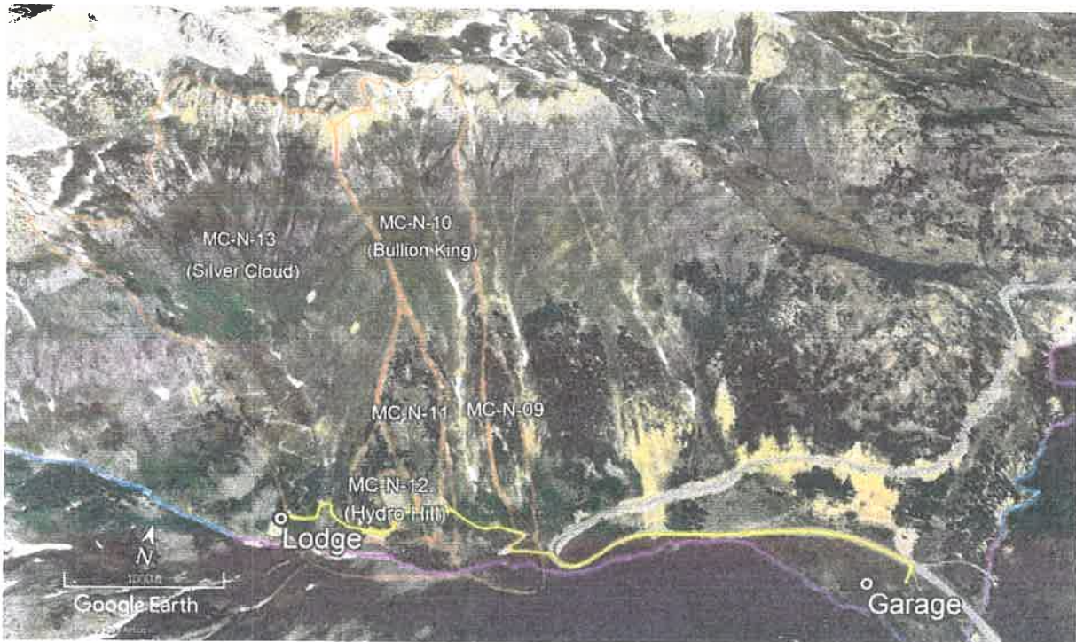
Figure 5. Avalanche terrain on the north side of Mill Creek affecting FSR 821. MC-N-10 (Bullion King) and MC-N-13 (Silver Cloud) frequently produce large destructive avalanches which reach the access road. The other three paths (MC-N-09, -11, and -12) are much smaller in scale.
