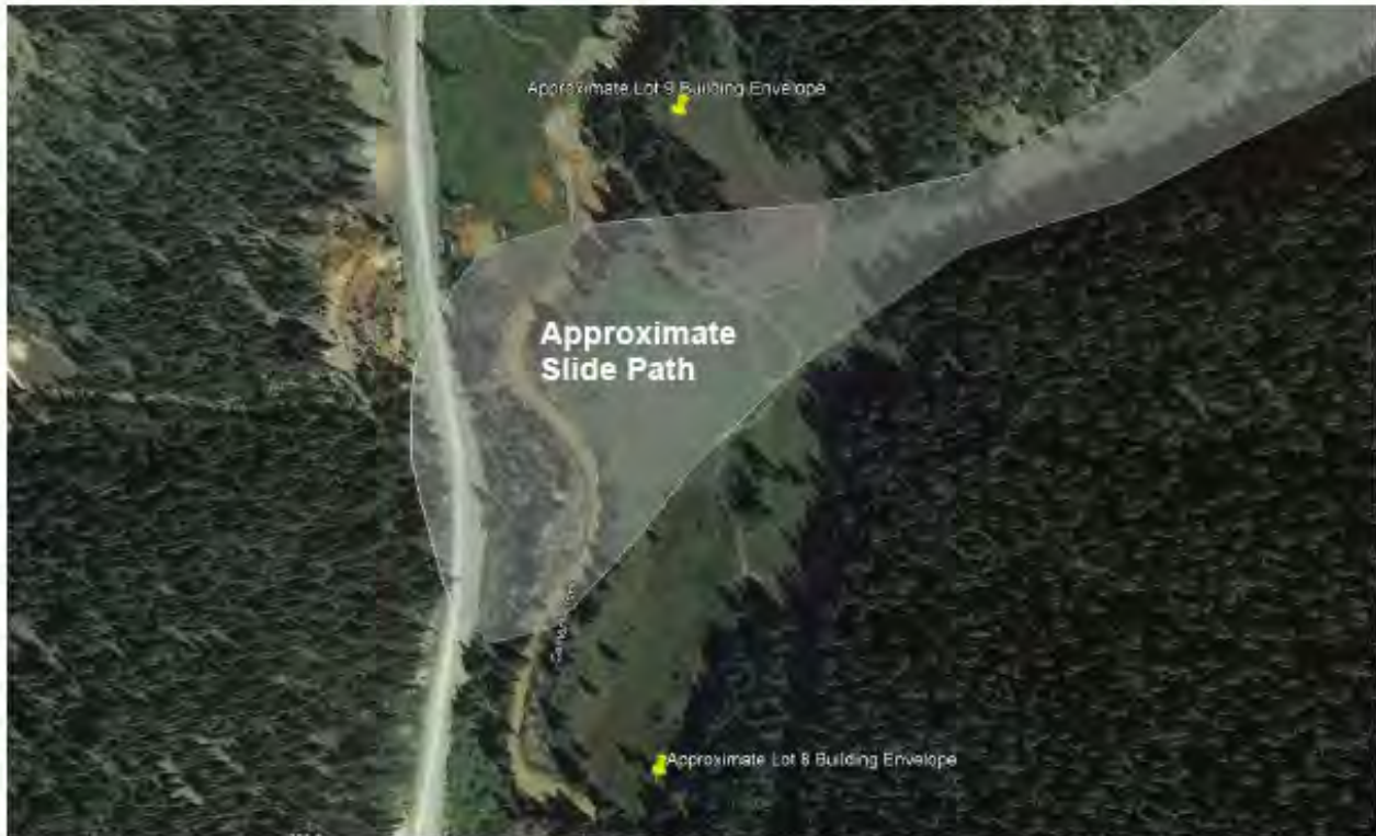
Figure 3.2: Schematic showing approximate relation of Lot 8 and 9 Building Envelopes to Grassy Gulch slide path. Location of slide path should be considered approximate and is based on interpretation of Avalanche Atlas drawing.
