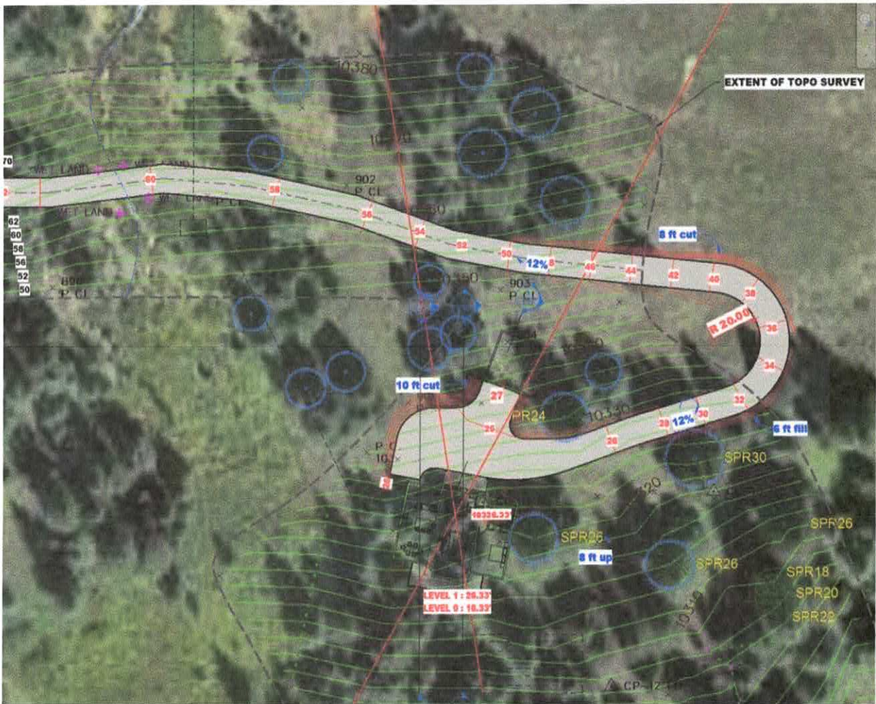
Satellite image with site plan overlaid. Note the location of trees relative to the structure. Those trees range from 30 to 60 feet tall and have been modeled into the following pictures.
